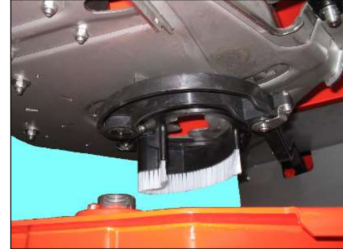
Drop Guide with disc removed
